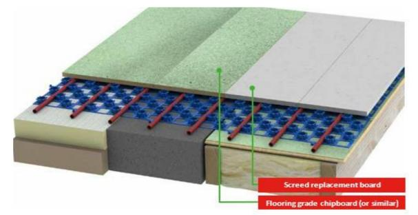
**PROFIX<sup>™</sup> PLUS - PIPE IN DIFFUSER PLATE SYSTEM** Suitable for 14mm to 17mm diameter pipe
